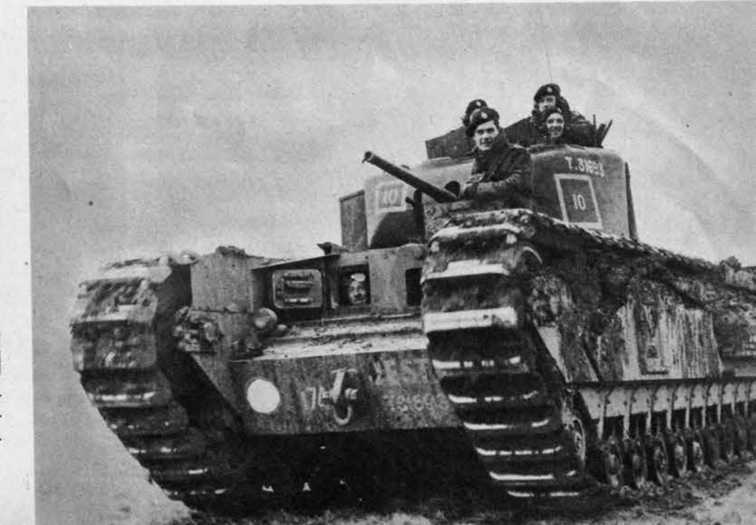
British Cromwell doesn't have T-34's wide track but has borrowed its five large wheels, high-set front idler and rear driving sprocket. Churchill (below) is unusual in having eleven small bogie wheels, very high rear sprocket and front idler, and long, overall tracks.
